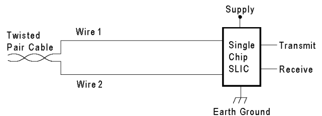
Fig. 9. SLIC circuit with no protection.
